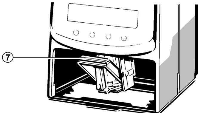
Dirt and dried up ink at the holder of the ink cartridge can be removed with a soft cleaning cloth moistened in spirit (see figure 2)
